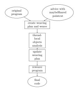
Figure 5: Weaving process for maybeShared pointcut
