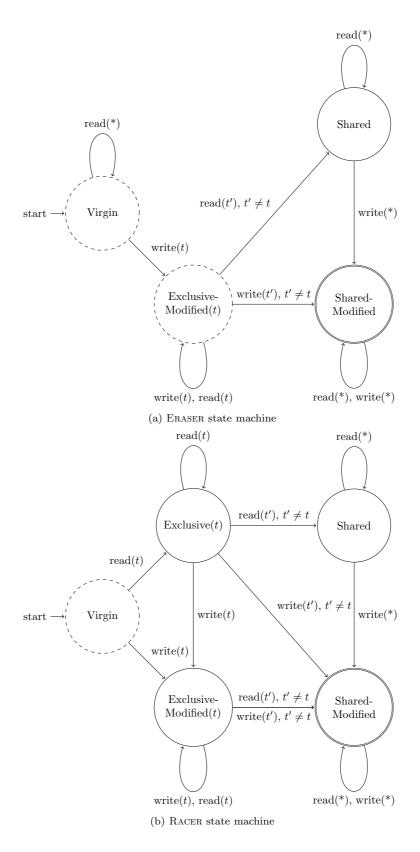
Figure 8: Eraser and Racer state machines; dashed states do no lock refinement; double-lined states report race potential
