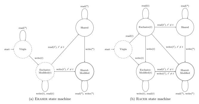
Figure 5: ERASER and RACER state machines; dashed states do no lock refinement; double-lined states report race potential
