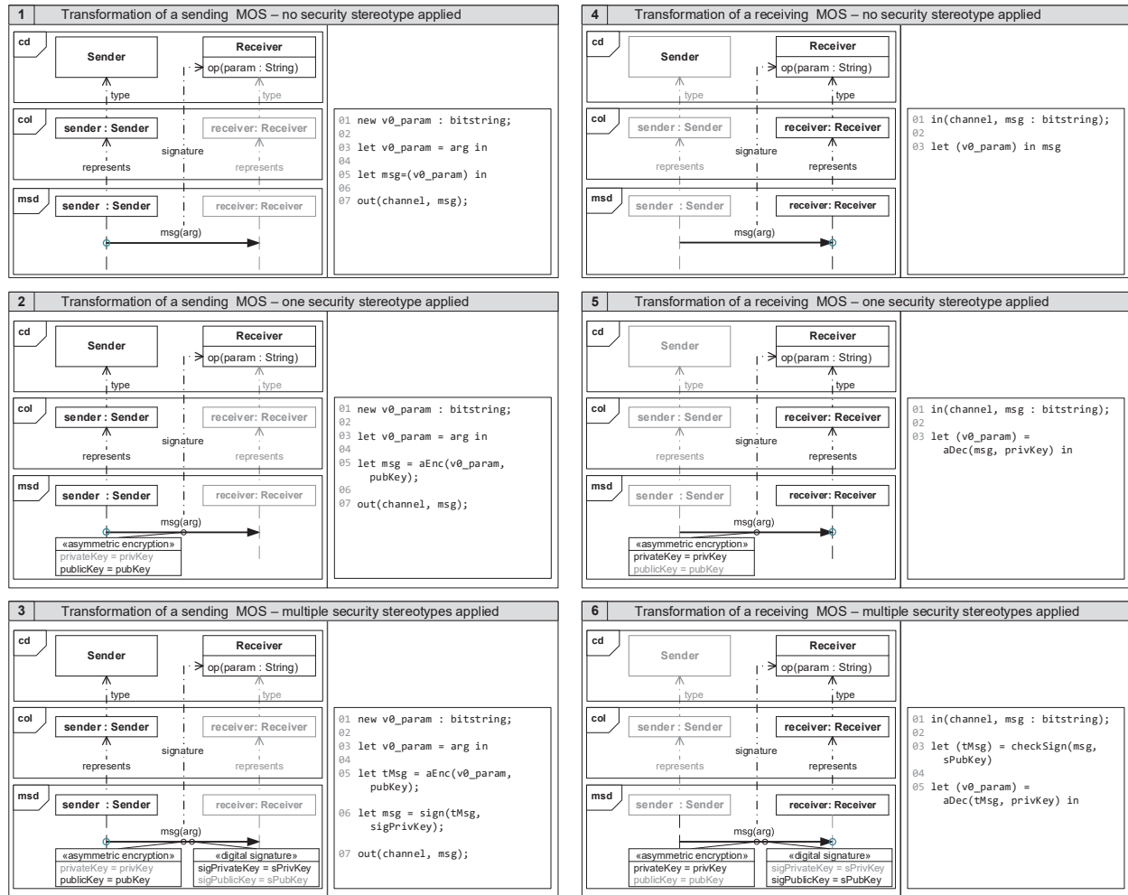
Figure 3: Transformation rules for the transformation from MSDs to ProVerif
